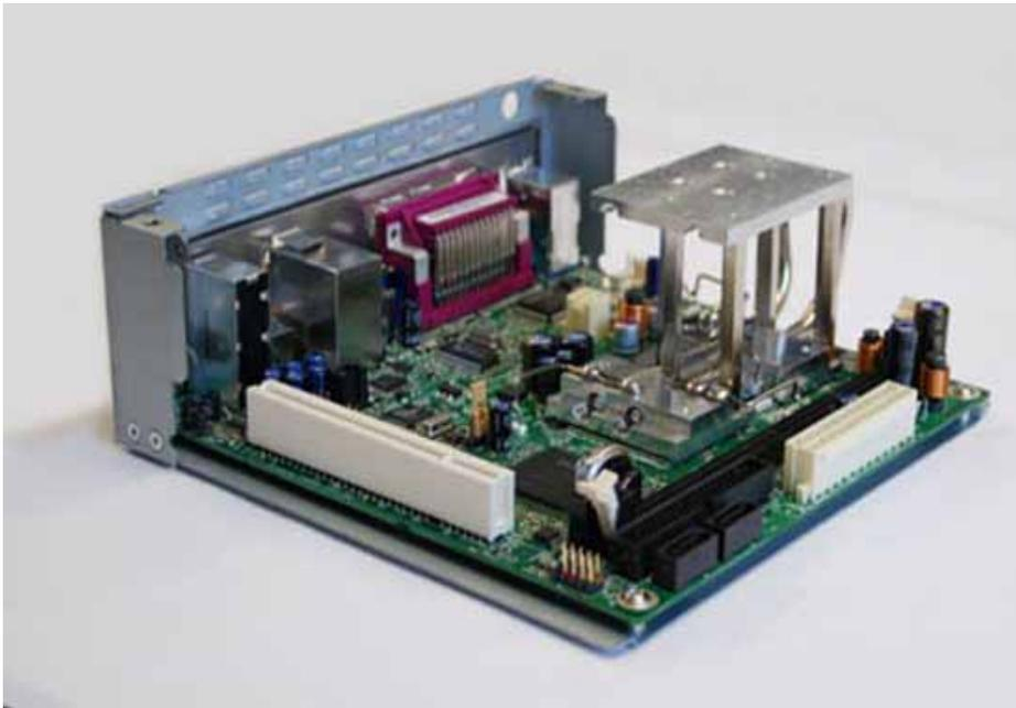
Remove the protective cover from the top of the heatsink/fan.
