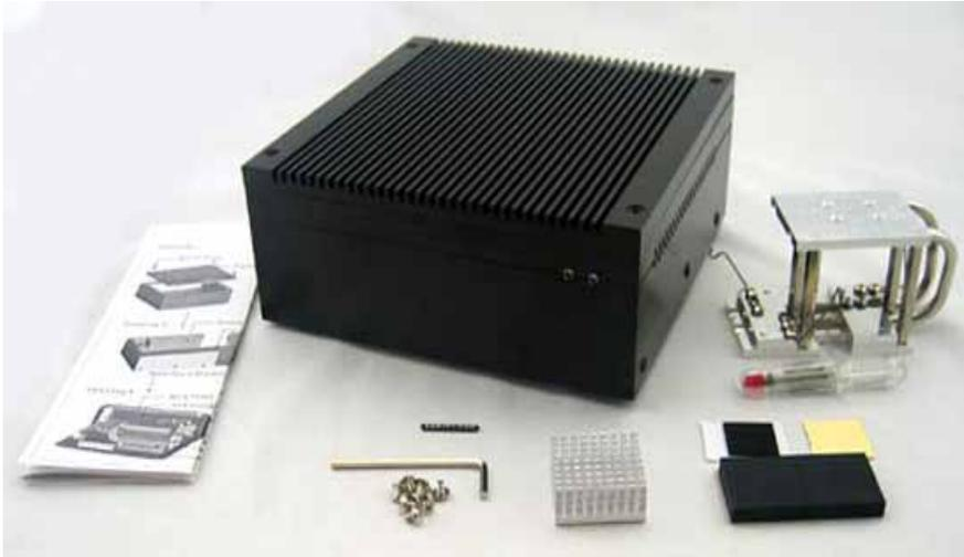
Open the top cover of the case with the wrench – part of the delivery content.
