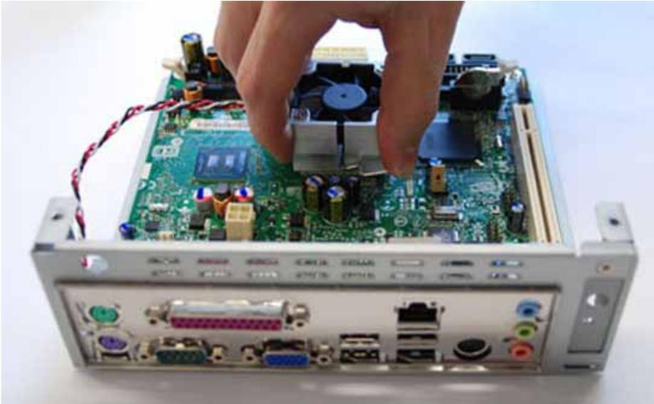
Clean the CPU (marked) and the chipset (marked).
